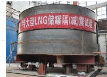
Seismic isolation model of nuclear power station
