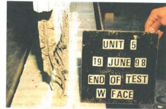
Figure 5.106. Unit 5 at end of test. Note buckled longitudinal bars.
