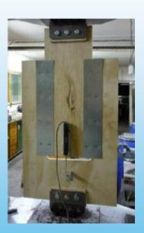
new plywood / stapled sheet metal blocking diaphragms
